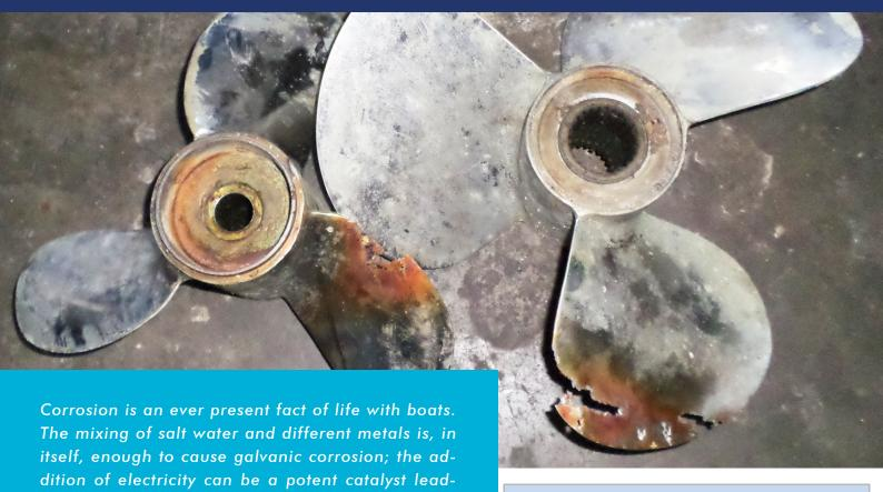
Your hull does not necessarily need to be metallic to suffer from the effects of galvanic or stray-current corrosion. Carbon fiber is a great conductor and even metallic components on fiberglass vessels such as propellers, shafts, drive units, rudder blades and skin fittings are also at risk.
