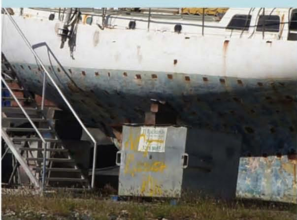
MAIN: Monohull hauled on hydraulic trailer. Large, adjustable pads support the hull on strong points. With the hull supported this way the keel is hanging, which allows inspection of the hull/keel joint if the boat is being surveyed.
