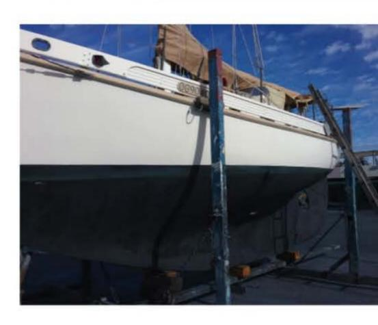
their keel, such as some modern racing yachts. Another disadvantage if the boat is being lifted for a survey is that, with the weight on the keel, it is not hanging for inspection of the keel-to-hull joint.
