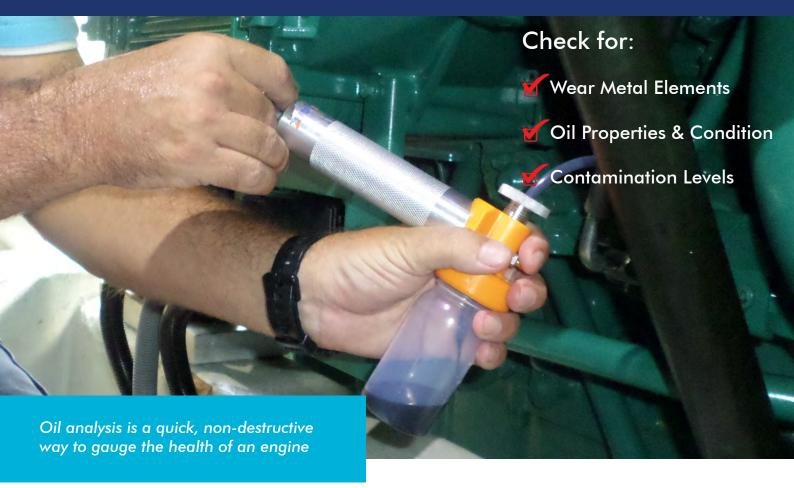
Oil Analysis provides vital information as to the condition of both the oil and the engine being tested. It can detect wear and contamination problems that, if left unchecked, can severely effect engine performance or cause engine failure.
