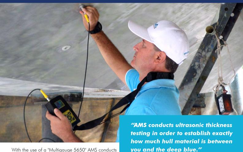
With the use of a "Multigauge 5650" AMS conducts ultrasonic thickness testing of metal and GRP hulls.
