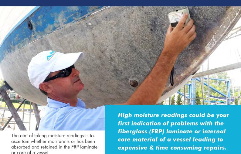
Persistently high moisture readings after the hull has had adequate time to dry may indicate the presence of "free" hygroscopic solutes within the laminate and accordingly may indicate a possible "Osmotic" condition before it becomes visible as blisters.
