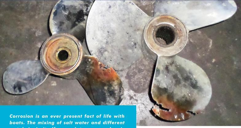
boats. The mixing of salt water and different metals is, in itself, enough to cause galvanic corrosion; the addition of electricity can be a potent catalyst leading to highly destructive stray-current corrosion
